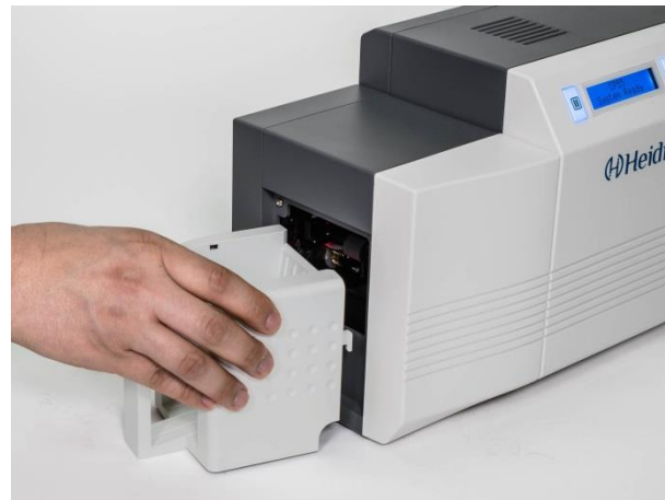
Figure 27 CP55 Dual installation of Rear Stacker
