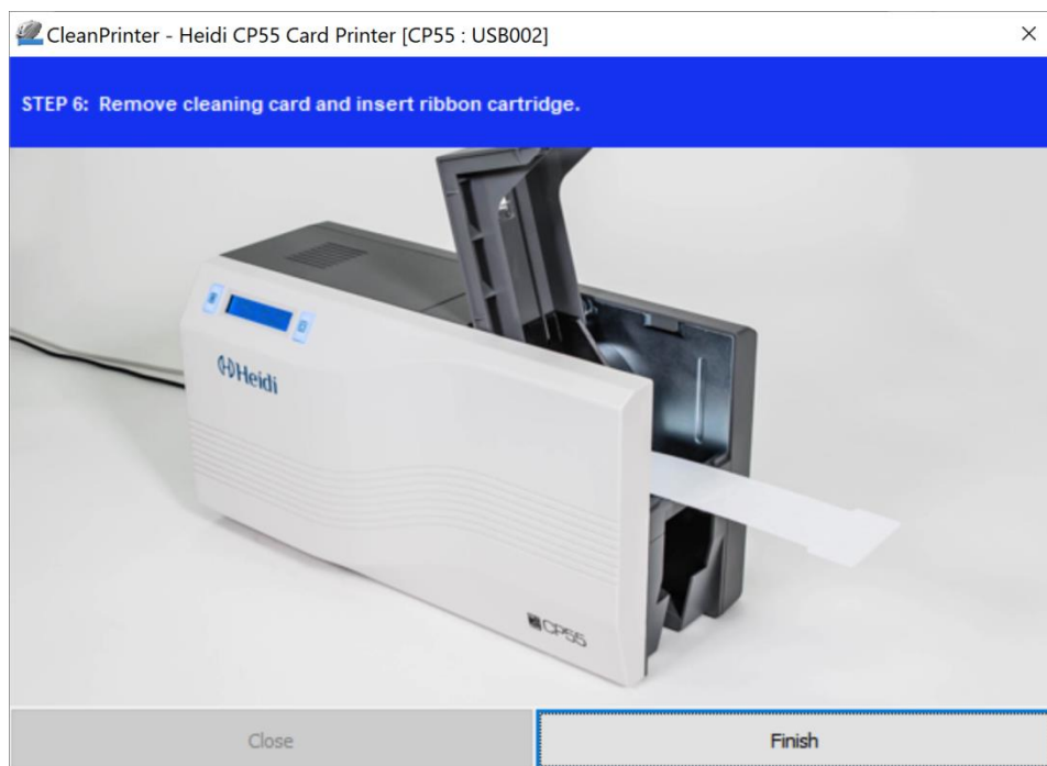
Figure 93 Printer cleaning Step 6
